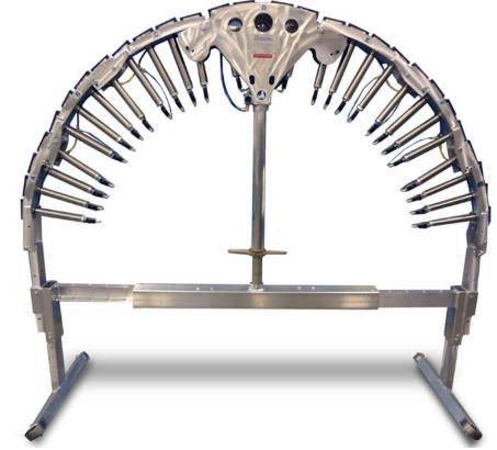
The Mini Econ-O-Ring (MECOR) is an adjustable, economically priced, small duty machine designed to service kilns with 1194mm – 2489mm (47"–98") Brick ID. The MECOR is single arched bricking machine with a single adjustable frame system that allows the MECOR to be adjusted to different diameter combinations within its range.
