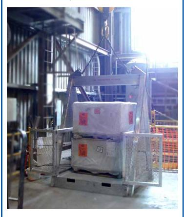
Safer than free lifting pallets with a crane. Keeps contents stable, secure, and contained.
