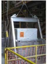
10,000 lb capacity. Load and unload up to 2 full pallets of bricks.
