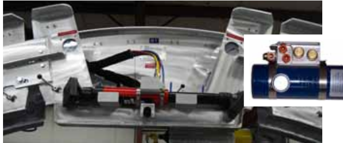
Pneumatic powered hydraulic jack with finger-tip controls
