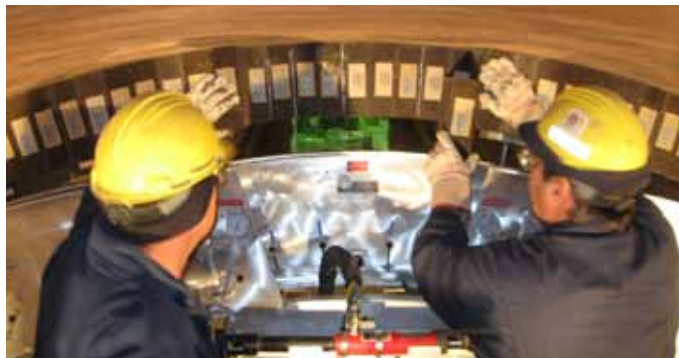
Open Keying section allows full easy access to holding arch
