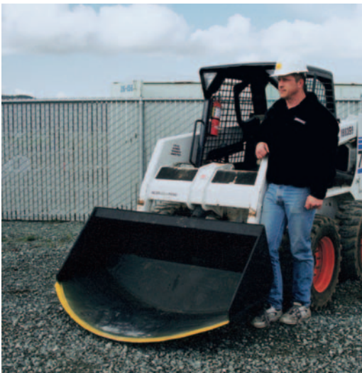
Radiused leading edge to penetrate rubble and reduce machine and operator impact.
