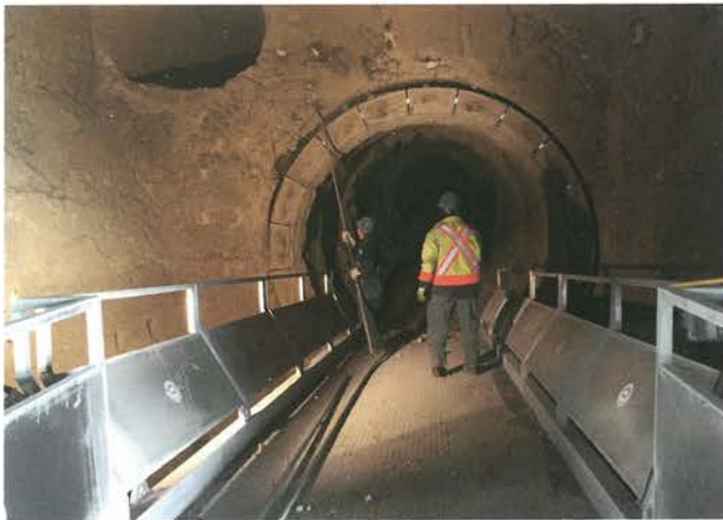
Kiln access ramps that are custom designed, modular, and made of lightweight aircraft aluminum, can be assembled as much as 40% faster than aftermarket or self-assembled ramps.
