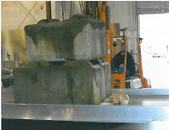
Kiln access ramp load testing.
