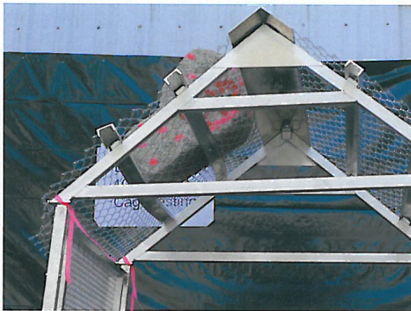
Safety inspection cage supporting simulated falling coating weighing 201 kg.
