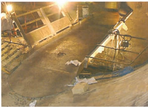
Figure 1. Lightweight kiln access ramp at Tilden/Cliffs Mines, Michigan, USA.
