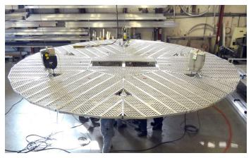
suspended by six 1,500-pound-capacity hoists, carries a four-person team, tools and materials up and down the 80-foot work area.
