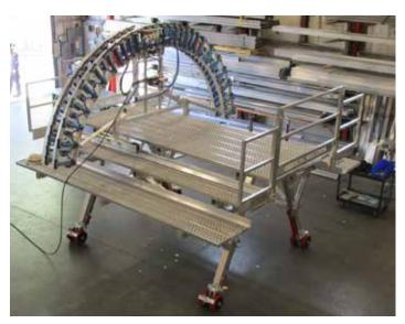
**STEP DECK OPTION** Step deck option gives workers more space moving materials underneath machine and can accommodate most fork truck access in larger size kilns.
