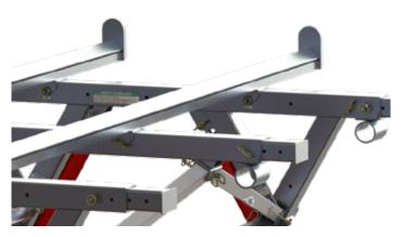
**PIN CONNECTIONS AND SYMMETRICAL PART DESIGN** Machine is assembled with pins connections, and symmetrical part designs allows assembly to be done without tools and under 2 hours. All components are modular and can fit through a 1M x 1M door
