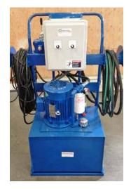
HYDRAULIC DRIVE 5-horsepower hydraulic drive moves material in either direction.
