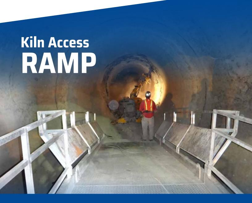
Access is the first consideration in Kiln Maintenance. The Kiln Access Ramps gets personnel and equipment in and out of the kiln safely
