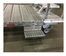
ERGONOMICALLY DESIGNED with steps so workers can access spring line of kiln easier and safer
