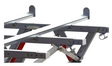
PIN CONNECTIONS AND SYMMETRICAL PART DESIGN Machine is assembled with pins connections, and symmetrical part designs allows assembly to be done without tools and under 1 hour. All components are modular and can fit through a 1M x 1M door
