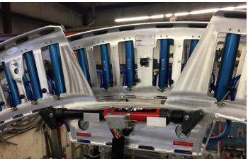
MASTER VALVE Dual master valves allows for Independent operation of cylinder or simultaneously controlled on both arches. KEYING JACK Keying Jack and air pressure gauge are standard
