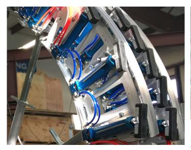
CYLINDER DESIGN Pneumatic valve in base cylinders with push-lock nickel plated brass fittings have articulating large rubber bumpers. The arch is an open design which allows for less than 10 minute cylinder change out.
