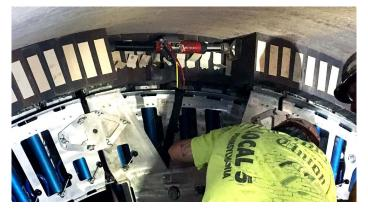
KEYING ACCESS Ergonomic Cut-Away Keying Section, exclusive to Bricking Solutions, give the key mason easy access to down kiln arch giving a clear view for critical key brick installation
