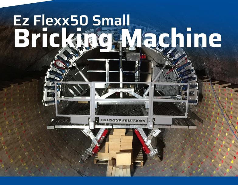
Same great machine in a compact size. Kilns 3-4 m (9' 10" - 13' 1") Brick ID 2640 mm - 3640mm This bricking machine has all the safety and efficiency features as the large size machine but it is designed for smaller kilns. This smaller machine has 3,000 kg load capacity and meets; CE, MSHA, CSA, and AWS safety standards.
