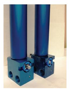
Both cylinders shown are 30mm. One cylinder with the new shaft and one with the old shaft.
