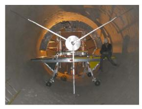
The laser target is a three armed self centering assembly that accurately centers the target on the centerline of the kiln. Please refer to separate set up directions provided with the unit. For burner tube adjustment using the laser slighter, the target assembly should be placed 25-30 yards/meters up the kiln from the laser beam source.
