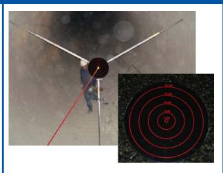
A target was the special equipment designed to be located in the middle of the kiln to receive a laser ray of a pointer being shot through the pipe of a burner or attached to a special fixture mounted on the nose of the burner. The target would be sturdy, easy to use, and able to withstand repeated use. The main target area was designed to be large and easy to see from a distance.
