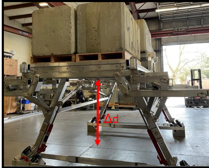
Figure 7. Deflection measurement point
