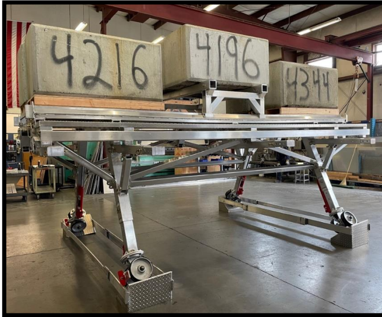
Figure 5. work platform frame with weigh blocks
