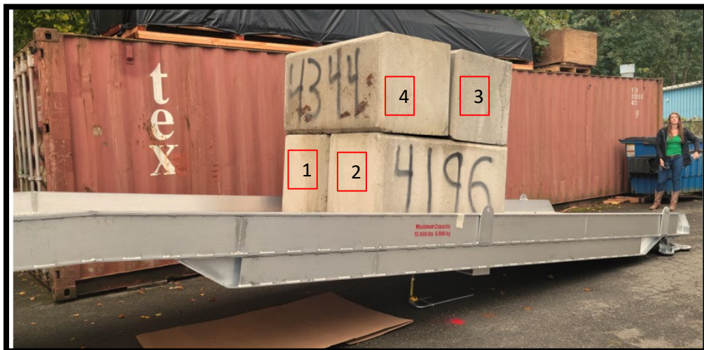
Figure 5: Blocks are labeled in the order it was loaded onto the ramp.
