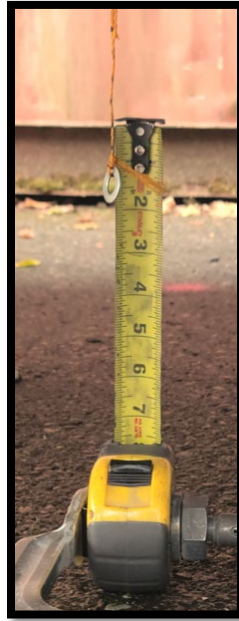
Figure 6: A string with a washer is attached to the I-beam, this allowed us to see deflection without going underneath the bridge while it was loaded.
