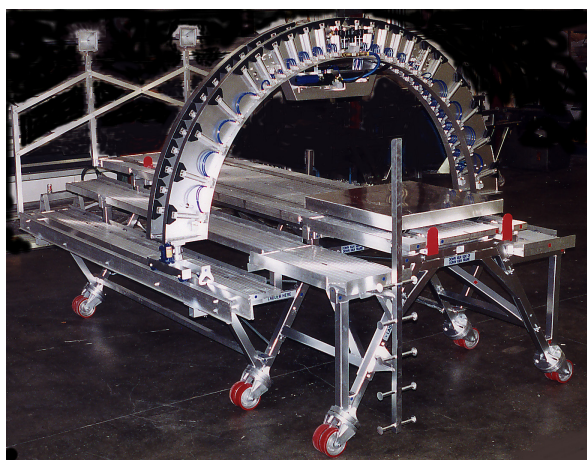
Photo 1: Modern Bricking Machine with trailer attachment. Trailer is used to increase weight capacity & work space. Facilitates simultaneous use of two shapes of brick during installation
