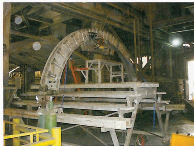
Figure 3. New Flat Deck Easy Flex FDMOR for the Lafarge Harleyville plant.
