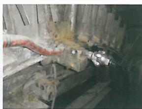
Poor maintenance of the machine – master valve failure.
