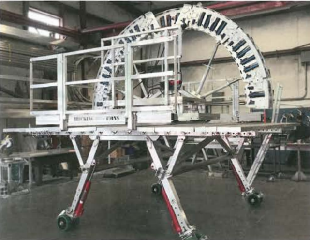
Bricking machines made from strong, yet lightweight, modular aluminum components can be installed by a skilled crew in just 60 – 90 min. as opposed to 6 – 8 hours for all-steel models.
